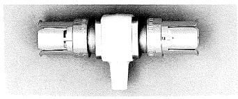
The VP-1 is a 50-ohm coaxial tee with GR fittings on each end and a plastic center collar. The collar is formed to provide a branch for insertion of P6034 10X or P6035 100X low-capacity, miniature passive probes. The VP-1 is designed for use with a Type 4S1, Type 4S2 or Type 3S76 Pulse-Sampling Plug-In Unit as a means of ac-
