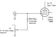
Schematic showing the Type Z Unit input modified to give an input resistance of 1000 megohms.
