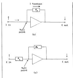
Figure 1. Conventional Operational Ampliplifier Symbols.
