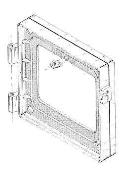
This modification is applicable to Tektronix camera-mounting bezels for Tektronix 5"-round-crt oscilloscopes\*. It installs a plastic mount which permits the use of a Tektronix rectangular polarized viewer (Part Number 016-039) when the camera is not in photographic position. Order through your Tektronix Field Engineer or local Field Office. Specify Tektronix Part Number 040-338. Price: \$0.35
