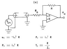
Lower power output required, reasonable signal/noise with currents to  $10^{-6}\ \text{amps}$  and negacycle bandwidth.
